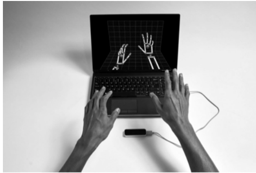
Figure 8. Detection of two hands by the Leap Motion
