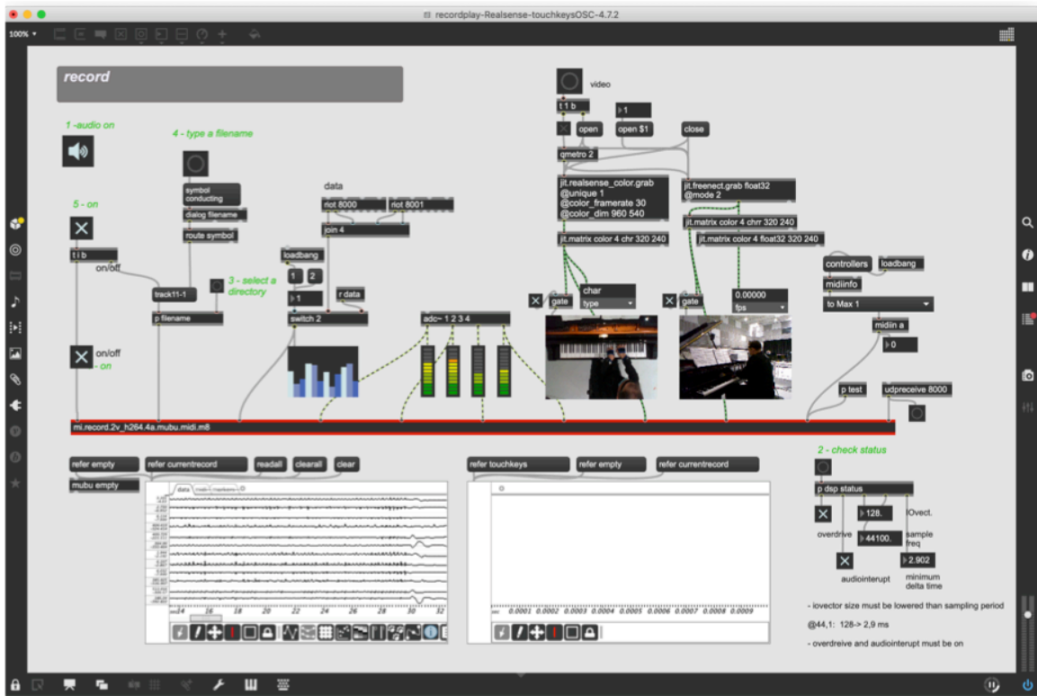
Figure 3. Patch in Max/MSP for recording audio, two Kinect videos, 3D acceleration and 3-axis gyrosopic data and MIDI.
